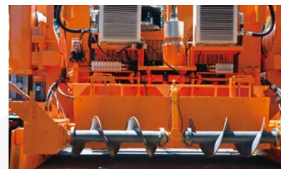
Scraping plate: Controlled by two hydraulic cylinders to control concrete quantity incoming to shaping-template, which could go up& down wholly or up& down independently at either left side or right side. 刮平板: 由两个液压缸控制, 控制混凝土进入成型模板的数量。该板可以整体升降, 也可以单独左边或右边升降。
