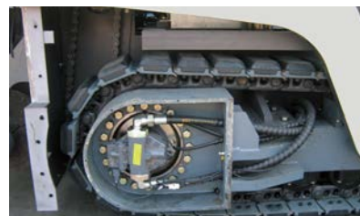
Travelling System: Two hydraulic-drive crawlers and microcomputer control ensure pre-set constant speed, correct straight-line running and smooth steering at bends. 行走装置: 两履带独立液压驱动, 微电脑控制, 能精确保证预选速度的恒定性, 准确的直线行驶性和平滑的弯道转向。
