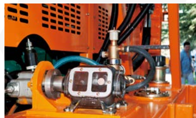
High Pressure Water Jet: To clean the machine effectively and prevent concrete from hardening freezing on machine. 高压水枪: 高压水枪能将整机有效冲洗干净, 防止混凝土凝固在机器上。
