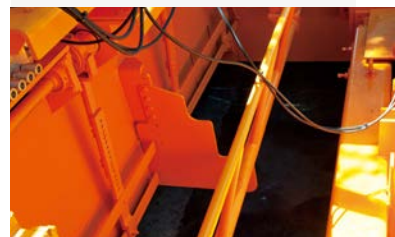
Tamper Bar: Multi-segments and multi-bars design to ensure further compacting and mud extraction. 捣固杆: 捣固杆是由多节组成, 多根垂杆悬挂, 能满足进一步密实和提浆要求。
