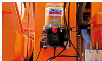
Centralized Lubrication: Can charge lubrication grease to high-temperature and motive components automatically, lengthen wear-out period effectively, greatly improve reliability of tamper and feeding. 集中润滑: 配有中央集中润滑系统, 高温、运动部位实现自动润滑。有效地延长了磨损周期, 大大提高了捣固、分料传动的可靠性。
