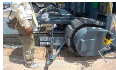
Bar inserted system: The trailing form with manual, air-powered bar insertion is designed to trail the track on two-track pavers. This system will accommodate most types of bars. 传力杆插入系统: 可通过手动或气动的方式将各种类型的传力杆插入混凝土。
